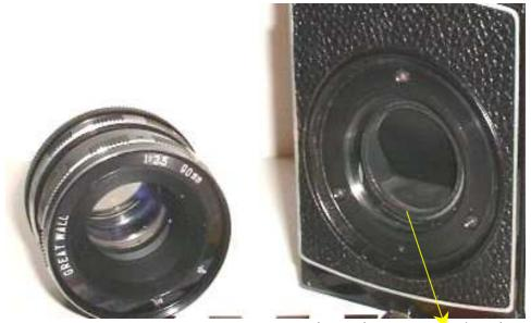
inner ring to protect the mirror-chamber
